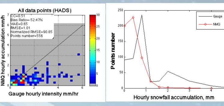
Left: The color-density scatterplot of SWE hourly accumulation of HADS SWE gauges and NMQ. The correlation coefficient, bias ratio, MAE, RMSE, Normalized RMSE (in %), and sample size are shown in the embedded text. Right: Histograms of HADS and NMQ hourly SWE for data shown in Fig. 3a.
