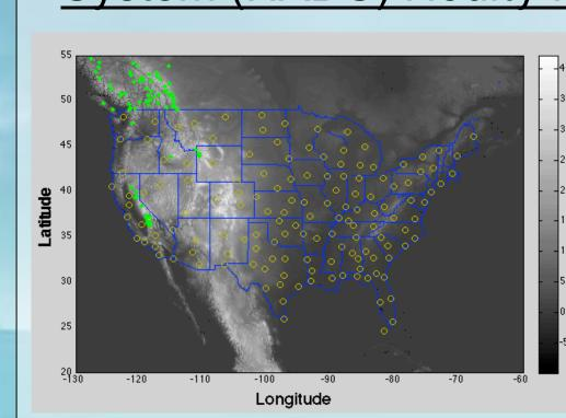
Locations of HADS gauges that transmit SWE information (green points), with terrain elevation (m) as background. The yellow circles indicate NEXRAD radar locations. 31 Canadian C-band radars are not included in this figure, but mosaicked by NMQ system.
